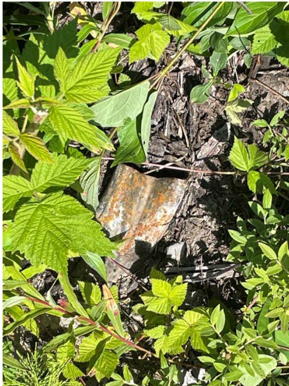
Figure 2-3. Left: Collar location of DDH NES26-27. Casing was damaged during egress of the drilling equipment from the site. Right: Collar location of DDH NES21-07 (Caracle Creek, 2026).
