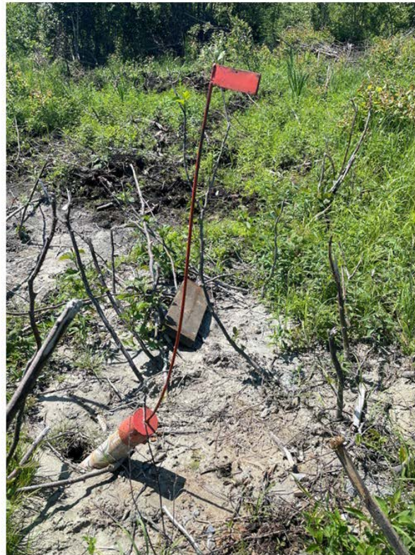
Figure 2-3. Left: Collar location of DDH NES26-27. Casing was damaged during egress of the drilling equipment from the site. Right: Collar location of DDH NES21-07 (Caracle Creek, 2026).
