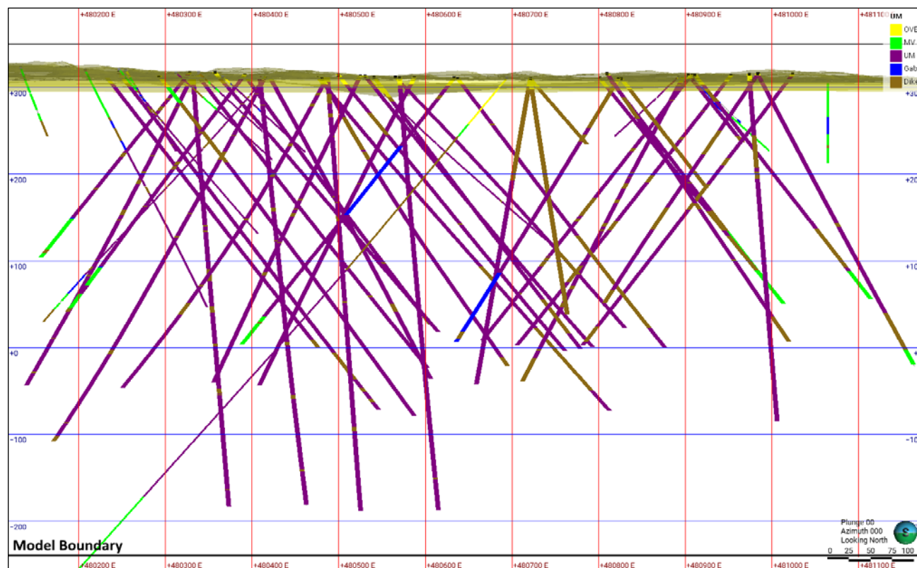
Figure 14-2. Longitudinal view (Looking North) of the Deloro Project showing the overburden volume (transparent yellow) as well as historical and CNC drill holes showing the main rock types, including the ultramafic package (UM) coloured in purple. Broader traces represent CNC holes while narrower ones are historical holes (Caracle Creek, 2026).
